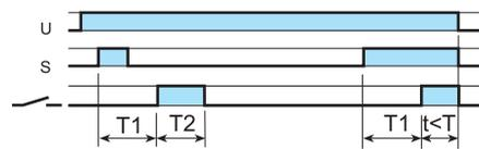
**(PE) Asymmetrical flasher (starting pulse off) with control signal.**
