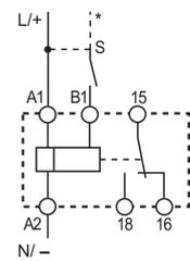
Wiring diagram (with control signal)
