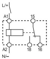
Wiring diagram (without control signal)
